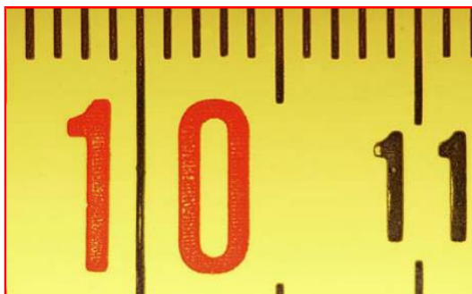
Fig. 5 Image of the millimeter rule (APS-C reflex + AF ED Micro-Nikkor 200 mm f/4D + Nikon 5T).
