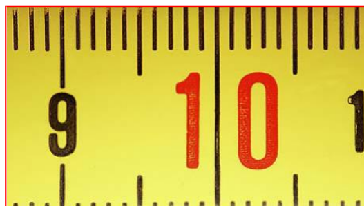
Fig. 3 Life-size image of a millimeter rule taken with APS-C (sensor size 15.7×23.6 mm) reflex camera.
